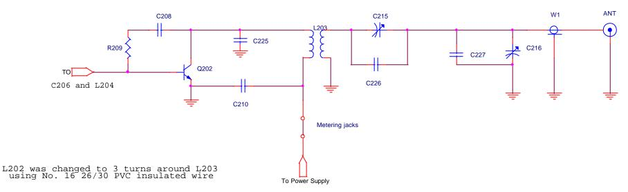
C225 was added. its value is selected for frequency, determine by inspection C226 and C227 are selected for frequency, determine by inspection.
